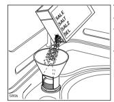
Then, using the funnel provided, pour in the salt until the container is full (approx. 1,5÷1,8 kg). Do not worry if water over flows from the unit when filling with salt this is quite normal.
